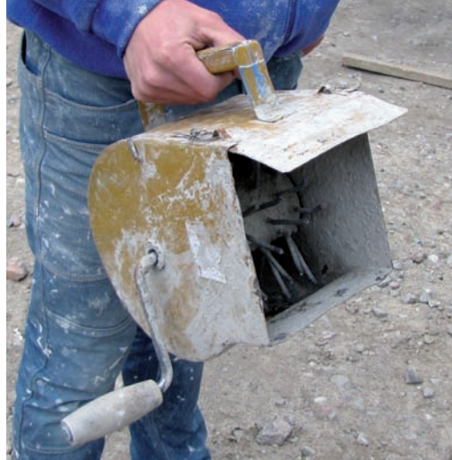
5. Tyrolean render applicator used to restore the façade in Gdynia
